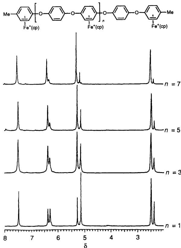
Fig. 3 Comparative NMR spectra (200 MHz, [[^2\text{H}_6]\text{dmso}] ) for complexes 27 ( n = 1 ), 52 ( n = 3 ), 55 ( n = 5 ) and 56 ( n = 7 )
